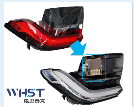
RL Prototype with integrated Rear Corner RADAR, hidden behind the lens
