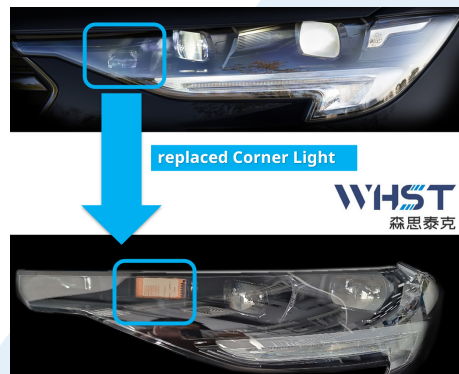
HL Prototype with integrated Front Corner RADAR
